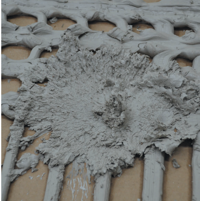
17 Clay crater created when air gap forces high air pressure onto surface of the clay.
